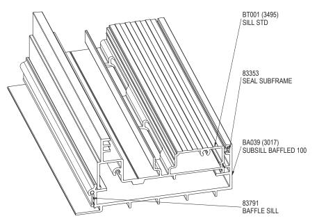
NOTE: IT IS MANDATORY THAT OPEN IN DOORS USING BT001 (3495) SILL STD USE BA039 (3017) SUBSILL BAFFLED 100, REFER TO COM-BD-06-30 FOR MACHINING DETAILS.
