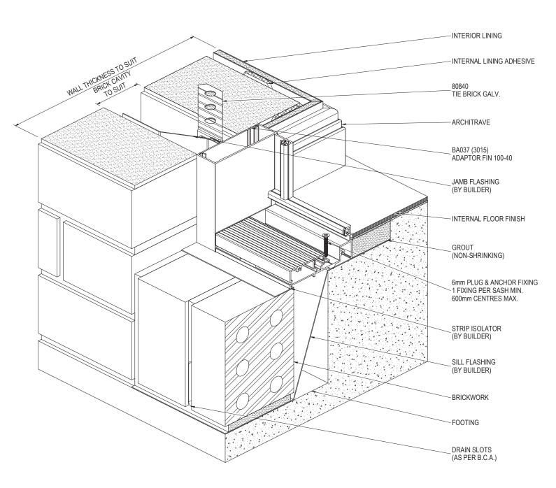
NOTE: FOR SITE CLASSIFICATIONS OF UP TO AND INCLUDING 'N6' OR SIMILAR, FIXINGS ARE TO BE AT 450mm CENTRE MAXIMUM, FOR SITUATIONS IN EXCESS OF THIS THE FIXINGS ARE TO BE AT 300mm CENTRES MAXIMUM. FIXING SIZE TO BE AS PER ENGINEER'S DETAILS.
