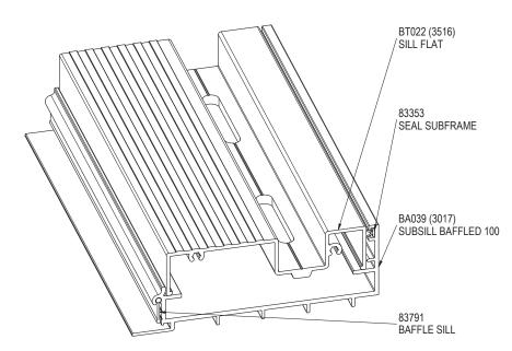
NOTE: IT IS RECOMMENDED THAT OPEN OUT & OPEN IN DOORS USING BT001 (3495) SILL STD USE BA039 (3017) SUBSILL BAFFLED 100, REFER TO COM-BD-06-31 FOR MACHINING DETAILS.
