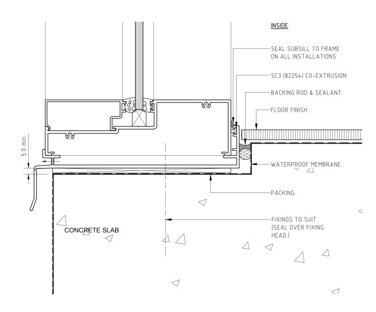
FIXINGS: TYPES & CENTRES TO BE PROJECT SPECIFIC. REFER TO SPECIFICATION &/OR COMPANY ENGINEER.
