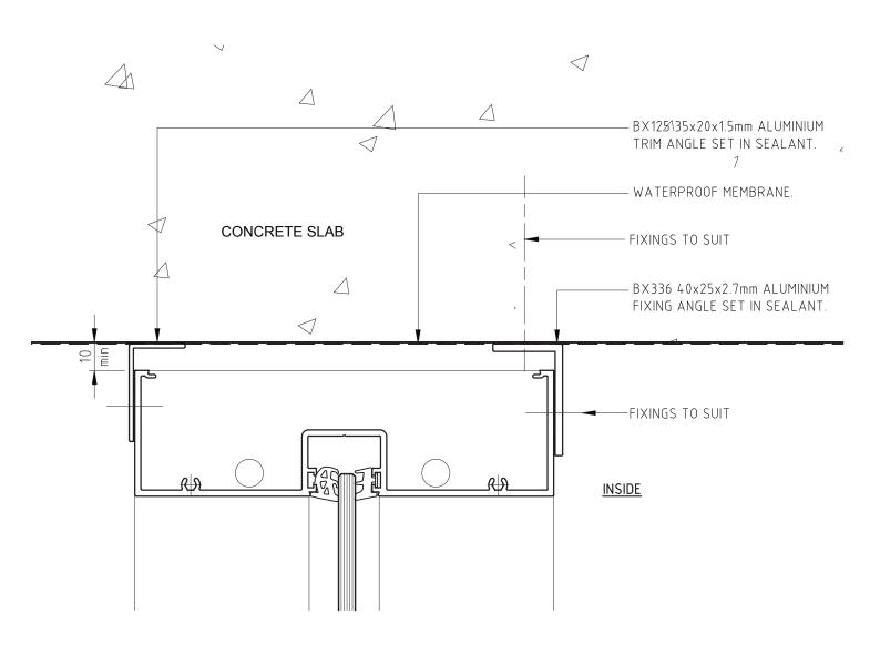
FIXINGS: TYPES & CENTRES TO BE PROJECT SPECIFIC. REFER TO SPECIFICATION &/OR COMPANY ENGINEER.
