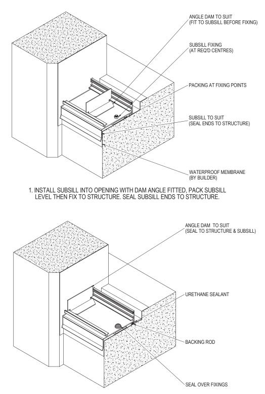
2: APPLY SEALANT TO VERTICAL FACE OF DAM ANGLE AND ALSO TO THE FLOOR OF THE SUBSILL, POSITION DAM ANGLE AGAINST STRUCTURE. SEAL ALL JOINTS BETWEEN ANGLE AND SUBSILL, SEAL ALL JOINTS BETWEEN ANGLE AND SUBSILL, SEAL OVER FIXINGS AND UNDER SUB SILL TO STRUCTURE.
