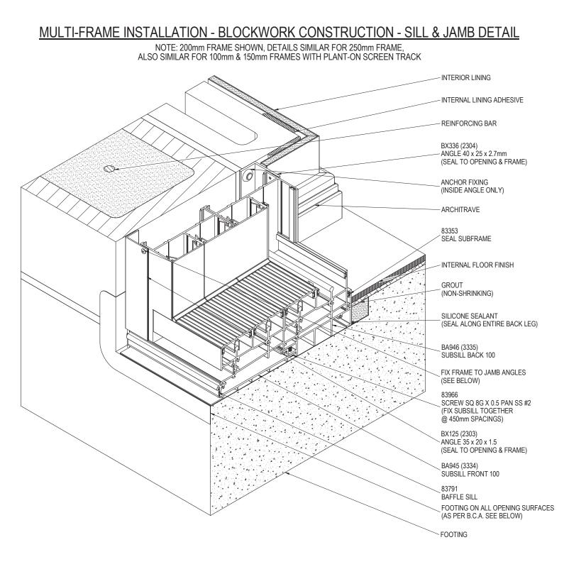
SURFACE OF BLOCKS TO DOOR / WINDOW OPENING MUST BE TANKED WITH A SUITABLE SEALER TO PREVENT INGRESS OF MOISTURE. ENSURE THAT THE SURFACES TO BE SEALED ARE SOUND, CLEAN, DRY AND FREE FROM ANY SURFACE CONTAMINANTS.
