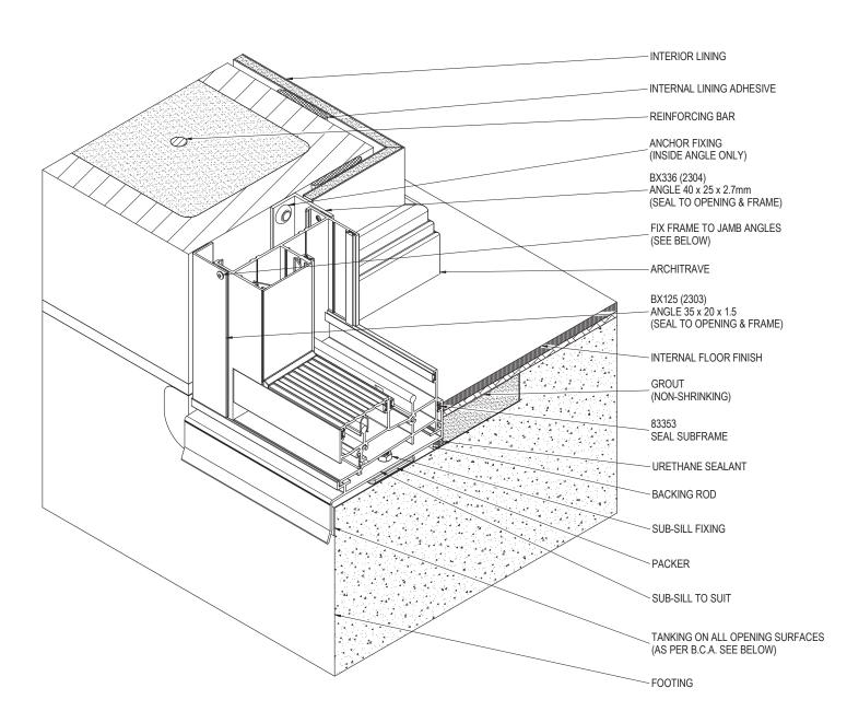
SURFACE OF BLOCKS TO DOOR / WINDOW OPENING MUST BE TANKED WITH A SUITABLE SEALER TO PREVENT INGRESS OF MOISTURE. ENSURE THAT THE SURFACES TO BE SEALED ARE SOUND, CLEAN, DRY AND FREE FROM ANY SURFACE CONTAMINANTS.
