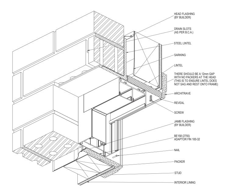
FIXINGS UP TO AND INCLUDING SITE CLASSIFICATION OF N6, C4 (3.0kPa) FIXINGS ARE TO BE AT 450mm CENTRE MAXIMUM. FOR SITUATIONS IN EXCESS OF THIS THE FIXINGS ARE TO BE AT 300mm CENTRES MAXIMUM. FIXING SIZE TO BE EQUIVALENT TO A Ø 2.2mm STEEL NAIL MIMIMUM.
