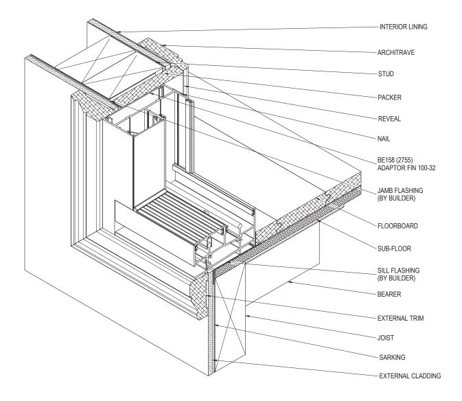
FIXINGS UP TO AND INCLUDING SITE CLASSIFICATION OF N6, C4 (3.0kPa) FIXINGS ARE TO BE AT 450mm CENTRE MAXIMUM. FOR SITUATIONS IN EXCESS OF THIS THE FIXINGS ARE TO BE AT 300mm CENTRES MAXIMUM. FIXING SIZE TO BE EQUIVALENT TO A  $\emptyset$  2.2mm STEEL NAIL MIMIMUM.
