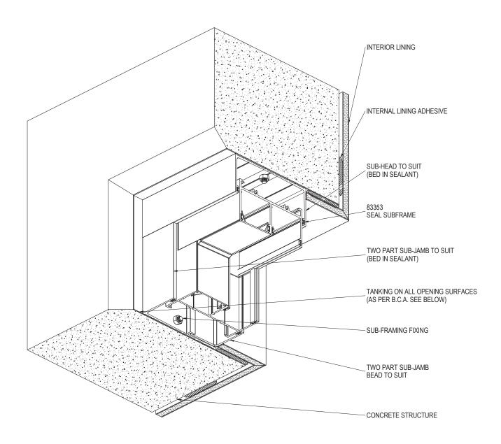
SURFACE OF BLOCKS TO DOOR / WINDOW OPENING MUST BE TANKED WITH A SUITABLE SEALER TO PREVENT INGRESS OF MOISTURE. ENSURE THAT THE SURFACES TO BE SEALED ARE SOUND, CLEAN, DRY AND FREE FROM ANY SURFACE CONTAMINANTS.
