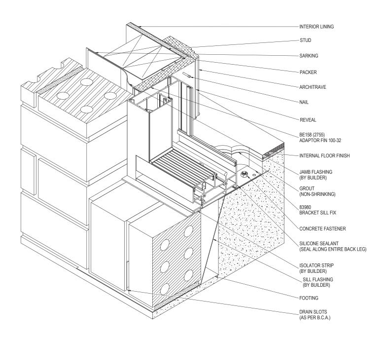
FIXINGS UP TO AND INCLUDING SITE CLASSIFICATION OF N6, C4 (3.0kPa) FIXINGS ARE TO BE AT 450mm CENTRE MAXIMUM. FOR SITUATIONS IN EXCESS OF THIS THE FIXINGS ARE TO BE AT 300mm CENTRES MAXIMUM. FIXING SIZE TO BE EQUIVALENT TO A Ø 2.2mm STEEL NAIL MIMIMUM.
