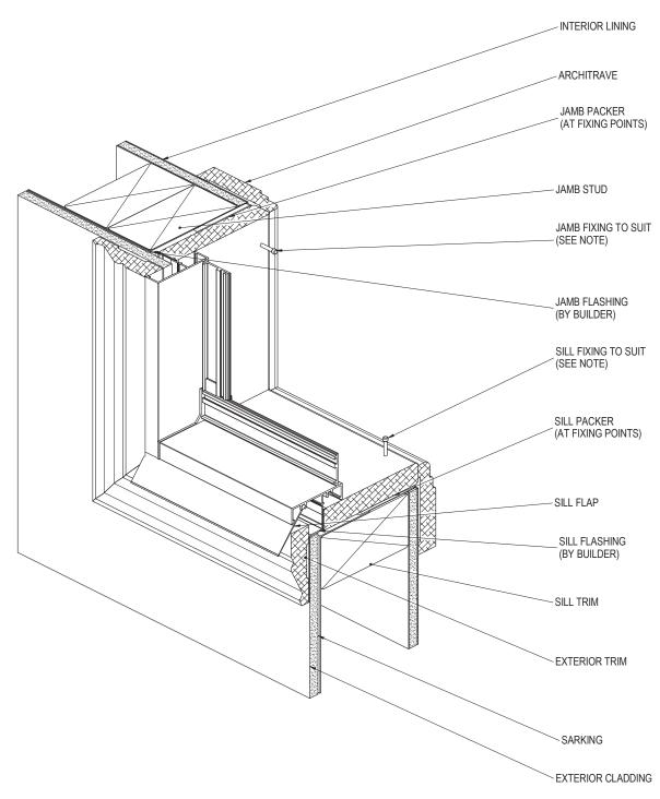
NOTE: FOR SITE CLASSIFICATIONS OF UP TO AND INCLUDING 'N6' OR SIMILAR, FIXINGS ARE TO BE AT 450mm CENTRE MAXIMUM, FOR SITUATIONS IN EXCESS OF THIS THE FIXINGS ARE TO BE AT 300mm CENTRES MAXIMUM. FIXING SIZE TO BE EQUIVALENT TO A  $\not\bigcirc$  2.2mm STEEL NAIL MIMIMUM.
