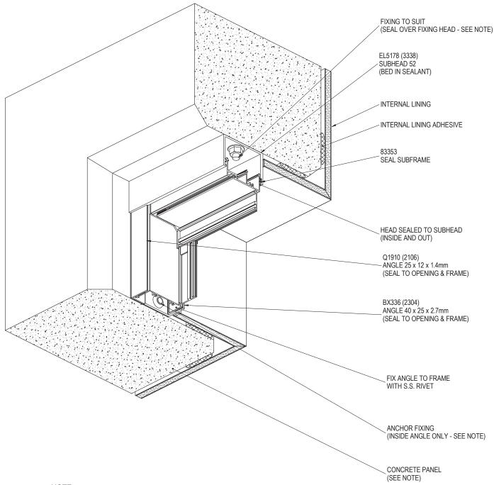
NOTE: SURFACE OF CONCRETE TO WINDOW OPENING MUST BE TANKED WITH A SUITABLE SEALER TO PREVENT INGRESS OF MOISTURE. ENSURE SURFACES TO BE SEALED ARE SOUND, CLEAN, DRY AND FREE FROM ANY CONTAMINANTS BEFORE SEALING.
