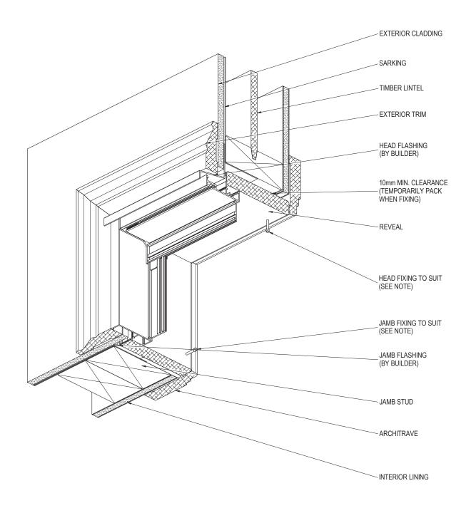
NOTE: FOR SITE CLASSIFICATIONS OF UP TO AND INCLUDING 'N6' OR SIMILAR, FIXINGS ARE TO BE AT 450mm CENTRE MAXIMUM, FOR SITUATIONS IN EXCESS OF THIS THE FIXINGS ARE TO BE AT 300mm CENTRES MAXIMUM. FIXING SIZE TO BE EQUIVALENT TO A  $\emptyset$ 2.2mm STEEL NAIL MIMIMUM.
