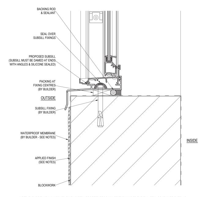
NOTE: ENSURE THAT ANY APPLIED FINISH DOES NOT RESTRICT DRAINAGE FROM UNDER THE SILL. SEAL COAT MUST OVERLAP END OF APPLIED FINISH TO SILL TANKING.
