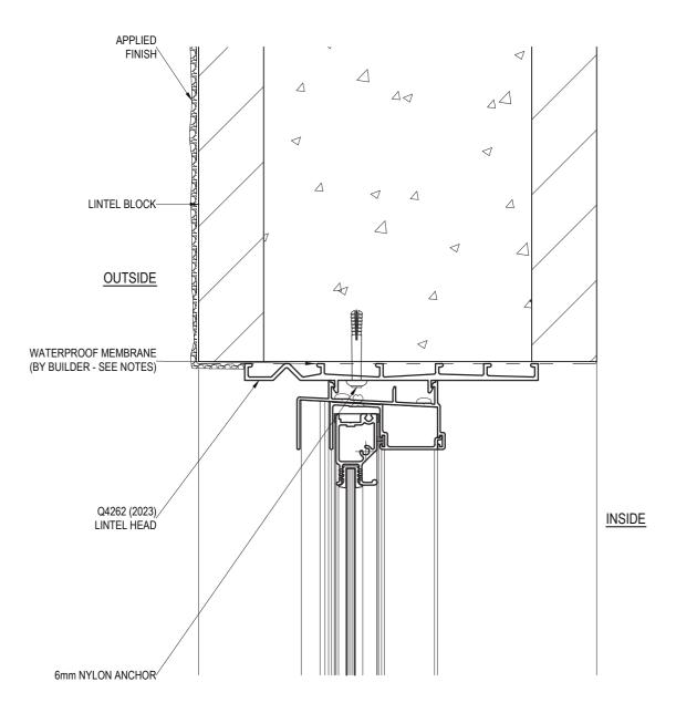
NOTE: SURFACE OF BLOCKS TO DOOR / WINDOW OPENING MUST BE TANKED WITH A SUITABLE SEALER TO PREVENT INGRESS OF MOISTURE. ENSURE MEMBRANE IS COMPATIBLE WITH A 1 PART POLYURETHANE SEALANT E.G. SIKAFLEX PRO 2HP.
