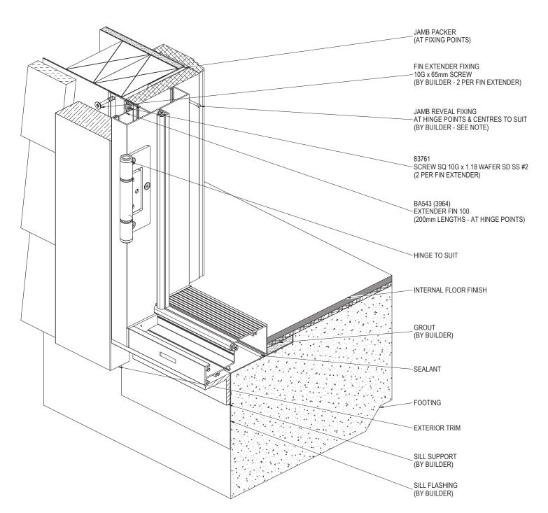
NOTE: FOR SITE CLASSIFICATIONS OF UP TO AND INCLUDING 'N6' OR SIMILAR, FIXINGS ARE TO BE AT 450mm CENTRE MAXIMUM, FOR SITUATIONS IN EXCESS OF THIS THE FIXINGS ARE TO BE AT 300mm CENTRES MAXIMUM. FIXING SIZE TO BE EQUIVALENT TO A otin 2.2mm STEEL NAIL MIMIMUM.
