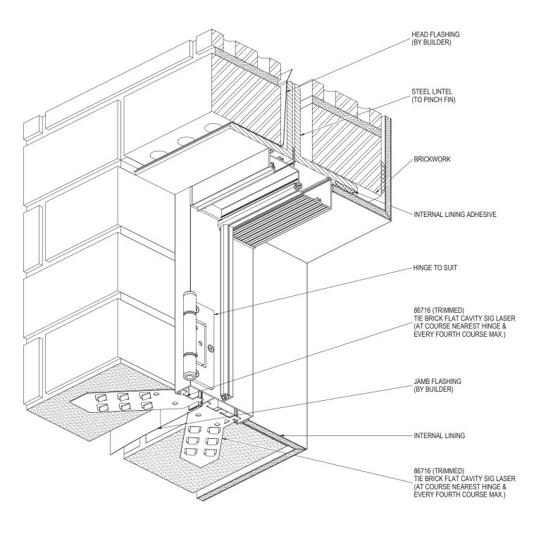
NOTE: FOR SITE CLASSIFICATIONS OF UP TO AND INCLUDING 'N6' OR SIMILAR, FIXINGS ARE TO BE AT 450mm CENTRE MAXIMUM, FOR SITUATIONS IN EXCESS OF THIS THE FIXINGS ARE TO BE AT 300mm CENTRES MAXIMUM. FIXING SIZE TO BE EQUIVALENT TO A  $\phi$  2.2mm STEEL NAIL MIMIMUM.
