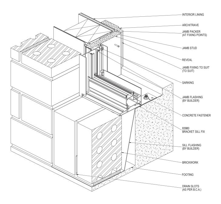
NOTE: FOR SITE CLASSIFICATIONS OF UP TO AND INCLUDING 'N6' OR SIMILAR, FIXINGS ARE TO BE AT 450mm CENTRE MAXIMUM, FOR SITUATIONS IN EXCESS OF THIS THE FIXINGS ARE TO BE AT 300mm CENTRES MAXIMUM. FIXING SIZE TO BE EQUIVALENT TO A  $\phi$ 2.2mm STEEL NAIL MIMIMUM.
