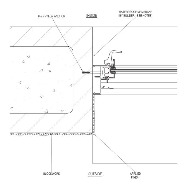
NOTE: SURFACE OF BLOCKS TO DOOR / WINDOW OPENING MUST BE TANKED WITH A SUITABLE SEALER TO PREVENT INGRESS OF MOISTURE. ENSURE MEMBRANE IS COMPATIBLE WITH A 1 PART POLYURETHANE SEALANT E.G. SIKAFLEX PRO 2HP.
