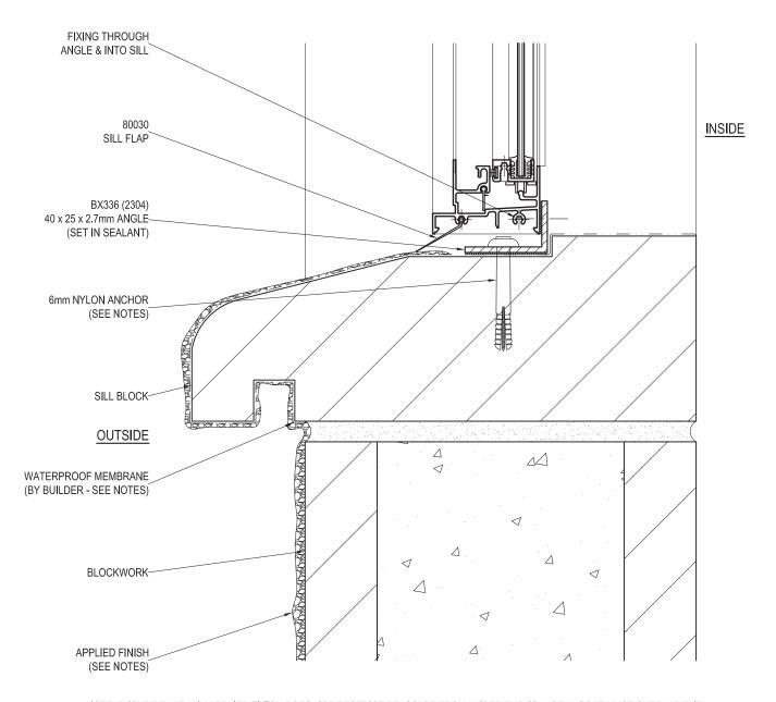
NOTE: ENSURE THAT ANY APPLIED FINISH DOES NOT RESTRICT DRAINAGE FROM UNDER THE SILL. SEAL COAT MUST OVERLAP END OF APPLIED FINISH TO SILL TANKING.
