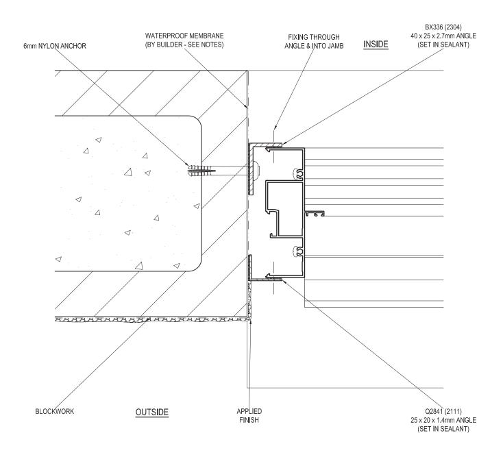
NOTE: SURFACE OF BLOCKS TO DOOR / WINDOW OPENING MUST BE TANKED WITH A SUITABLE SEALER TO PREVENT INGRESS OF MOISTURE. ENSURE MEMBRANE IS COMPATIBLE WITH A 1 PART POLYURETHANE SEALANT E.G. SIKAFLEX PRO 2HP.
