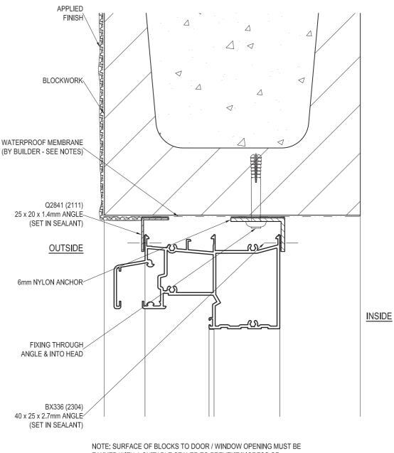
TANKED WITH A SUITABLE SEALER TO PREVENT INGRESS OF MOISTURE. ENSURE MEMBRANE IS COMPATIBLE WITH A 1 PART POLYURETHANE SEALANT E.G. SIKAFLEX PRO 2HP.
