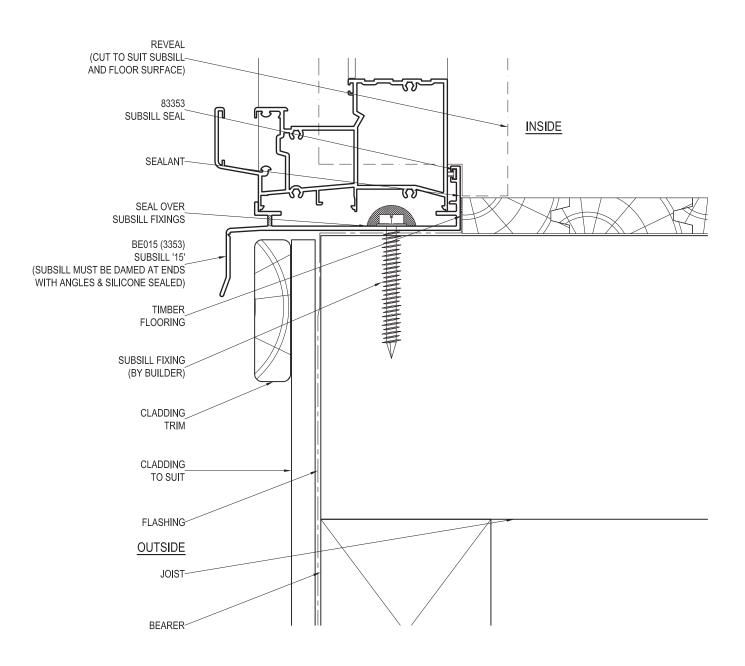
FIXINGS: UP TO AND INCLUDING SITE CLASSIFICATION OF N6, C4 (3.0 kPa) FIXINGS ARE TO BE AT 450mm CENTRE MAXIMUM. FOR SITUATIONS IN EXCESS OF THIS THE FIXINGS ARE TO BE AT 300mm CENTRES MAXIMUM. FIXING SIZE TO BE EQUIVALENT TO A Ø2.2mm STEEL NAIL MINIMUM.
