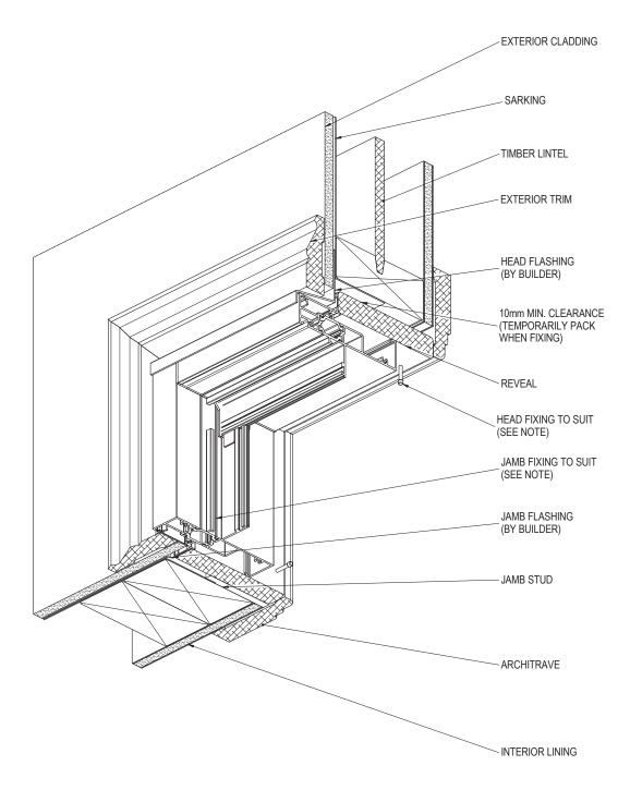
NOTE: FOR SITE CLASSIFICATIONS OF UP TO AND INCLUDING 'N6' OR SIMILAR, FIXINGS ARE TO BE AT 450mm CENTRE MAXIMUM, FOR SITUATIONS IN EXCESS OF THIS THE FIXINGS ARE TO BE AT 300mm CENTRES MAXIMUM. FIXING SIZE TO BE EQUIVALENT TO A  $\oslash$  2.2mm STEEL NAIL MIMIMUM.
