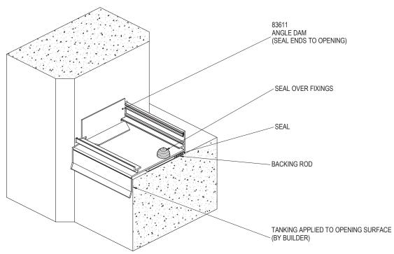
2. APPLY SEALANT TO VERTICAL FACE OF DAM ANGLE AND ALSO TO THE FLOOR OF THE SUBSILL. POSITION DAM ANGLE AGAINST THE STRUCTURE. SEAL ALL JOINTS BETWEEN THE ANGLE AND SUBSILL. SEAL ALL JOINTS BETWEEN ANGLE AND SUBSILL. SEAL OVER FIXINGS AND UNDER SUB SILL TO STRUCTURE.
