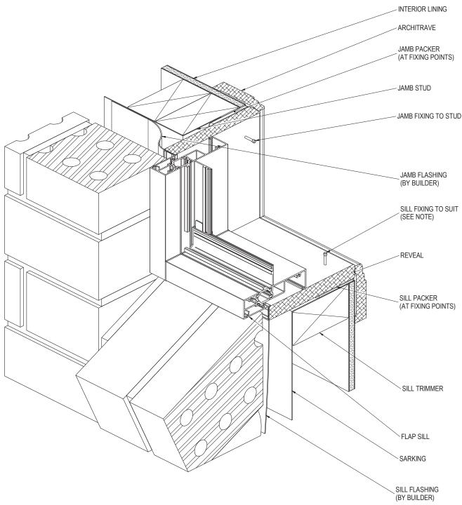
NOTE: FOR SITE CLASSIFICATIONS OF UP TO AND INCLUDING 'N6' OR SIMILAR, FIXINGS ARE TO BE AT 450mm CENTRE MAXIMUM, FOR SITUATIONS IN EXCESS OF THIS THE FIXINGS ARE TO BE AT 300mm CENTRES MAXIMUM. FIXING SIZE TO BE EQUIVALENT TO A  $\oslash$  2.2mm STEEL NAIL MIMIMUM.
