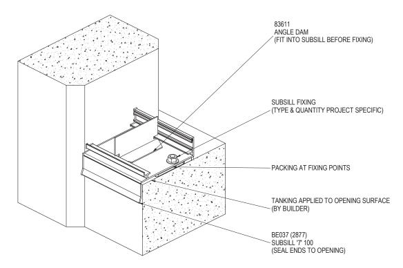
1. INSTALL SUBSILL INTO OPENING WITH DAM ANGLE FITTED. PACK SUBSILL LEVEL THEN FIX TO STRUCTURE. SEAL SUBSILL ENDS TO STRUCTURE.
