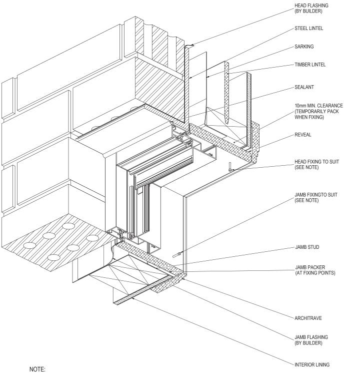
FOR SITE CLASSIFICATIONS OF UP TO AND INCLUDING 'N6' OR SIMILAR, FIXINGS ARE TO BE AT 450mm CENTRE MAXIMUM, FOR SITUATIONS IN EXCESS OF THIS THE FIXINGS ARE TO BE AT 300mm CENTRES MAXIMUM. FIXING SIZE TO BE EQUIVALENT TO A  $\oslash$  2.2mm STEEL NAIL MIMIMUM.
