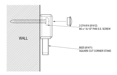
FIX SCREWS INTO PLASTER BOARD, USE WALL PLUGS INTO BRICK BEFORE SECURING SCREW. PLACE CAP ON CORNER.
