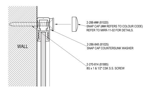
FIX SCREWS INTO PLASTER BOARD, USE SNAP CAPS TO HIDE FIXINGS. SECURE SCREWS AT 800mm CENTRES MAXIMUM ALONG ENTIRE FRAME.
