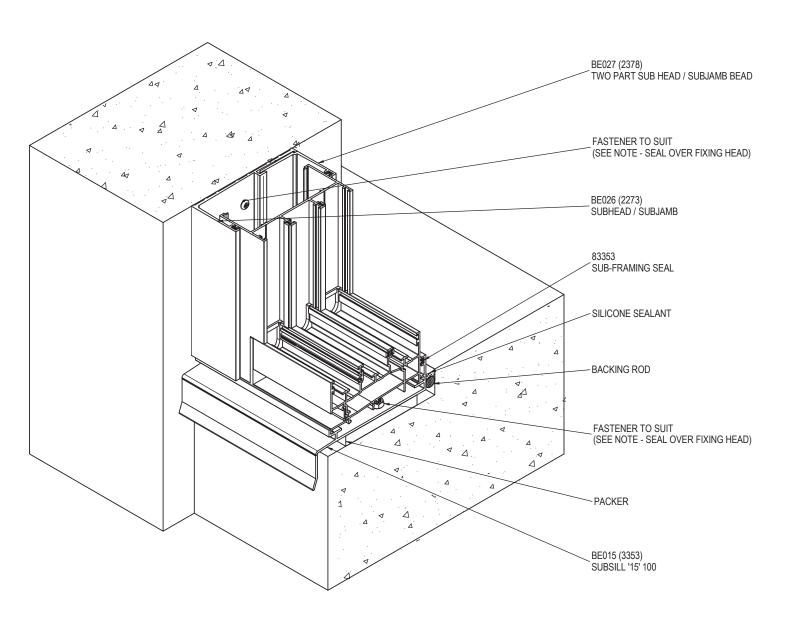
FIXINGS TYPES AND CENTRES TO BE PROJECT SPECIFIC. REFER TO SPECIFICATION &/OR COMPANY ENGINEER.
