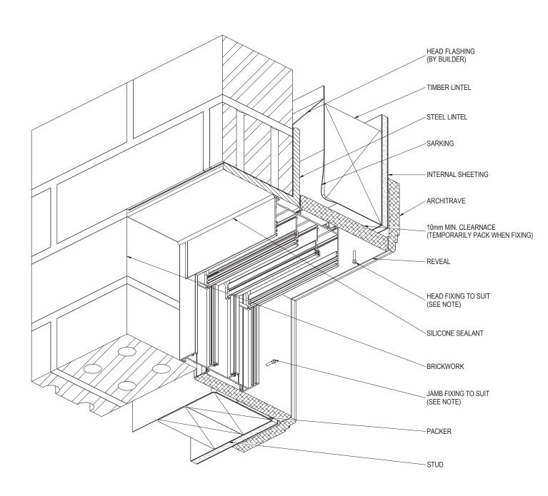
FOR SITE CLASSIFICATIONS OF UP TO AND INCLUDING 'N6' OR SIMILAR, FIXINGS ARE TO BE AT 450mm CENTRE MAXIMUM, FOR SITUATIONS IN EXCESS OF THIS THE FIXINGS ARE TO BE AT 300mm CENTRES MAXIMUM. FIXING SIZE TO BE EQUIVALENT TO A  $\, \phi$  2.2mm STEEL NAIL MIMIMUM.
