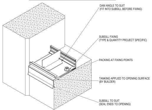
1. INSTALL SUBSILL INTO OPENING WITH DAM ANGLE FITTED. PACK SUBSILL LEVEL THEN FIX TO STRUCTURE. SEAL SUBSILL ENDS TO STRUCTURE.
