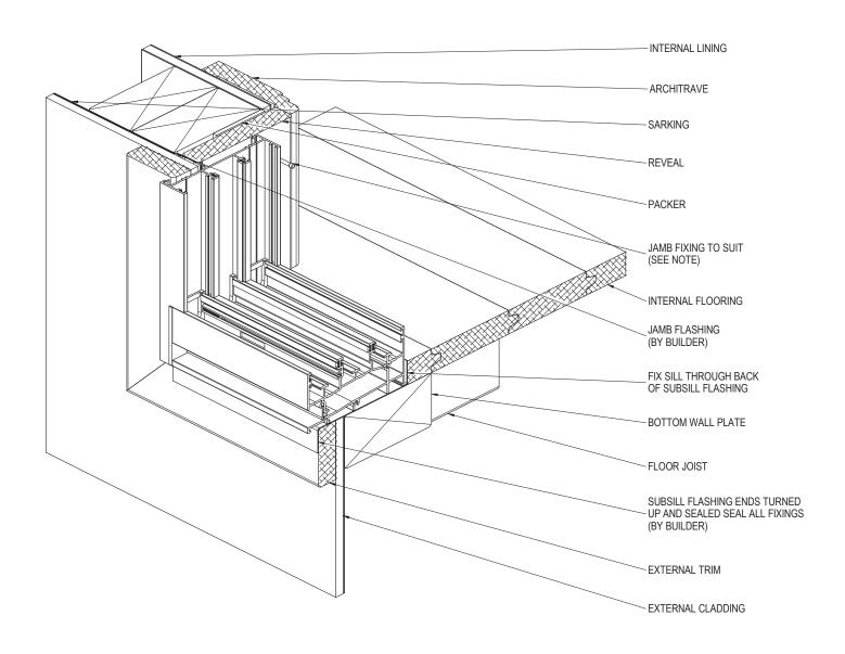
FOR SITE CLASSIFICATIONS OF UP TO AND INCLUDING 'N6' OR SIMILAR, FIXINGS ARE TO BE AT 450mm CENTRE MAXIMUM, FOR SITUATIONS IN EXCESS OF THIS THE FIXINGS ARE TO BE AT 300mm CENTRES MAXIMUM. FIXING SIZE TO BE EQUIVALENT TO A  $\oslash$  2.2mm STEEL NAIL MIMIMUM.
