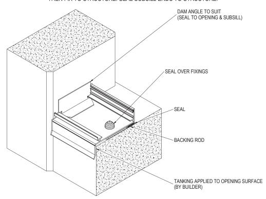
2.APPLY SEALANT TO VERTICAL FACE OF DAM ANGLE AND ALSO TO THE FLOOR OF THE SUBSILL. POSITION DAM ANGLE AGAINST STRUCTURE. SEAL ALL JOINTS BETWEEN ANGLE AND SUBSILL. SEAL ALL JOINTS BETWEEN ANGLE AND SUBSILL. SEAL OVER FIXINGS AND UNDER SUB SILL TO STRUCTURE.
