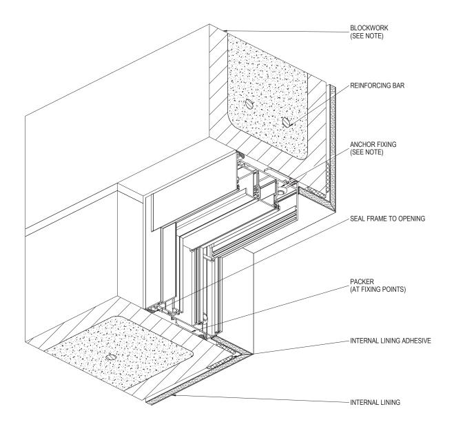
SURFACE OF BLOCKS TO WINDOW OPENING MUST BE TANKED WITH A SUITABLE SEALER TO PREVENT INGRESS OF MOISTURE. ENSURE SURFACES TO BE SEALED ARE SOUND, CLEAN, DRY AND FREE FROM ANY CONTAMINANTS BEFORE SEALING.
